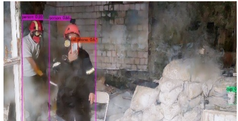
Object detection in smoke: with dehazing pre-processing
