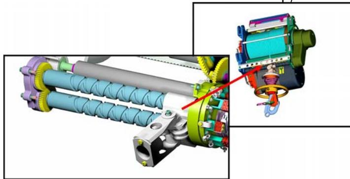
*Translating Drum Design-* The hoist cable drum moves back and forth in relation to a fixed position cable levelwind.
